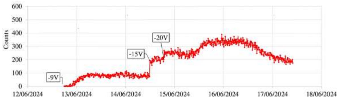
Figure 8. The measurement results of the constructed radon detection system for three different values of biasing voltage.
